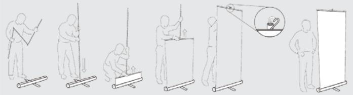
Less than 30 seconds for a quick setup solution. Unfold the tri-fold bar, insert the tri-fold bar into it's slot on the banner stand. Pull out the graphic while holding on to the tri-fold bar. Slightly tilt the banner stand to reach the top of pole and insert the hook into the top of tri-fold bar.
